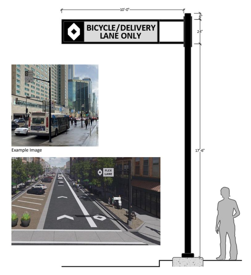
Description: Steel pole with "Bicycle /Delivery Lane Only" sign attached to tubular steel frame Signs to be according to Section 1091 – Sign Face, Sign Legend, and Supplemental Panels and Sign Posts to be according to Section 1093 – Sign Supports of the IDOT Standard Specifications<sup>32</sup>
