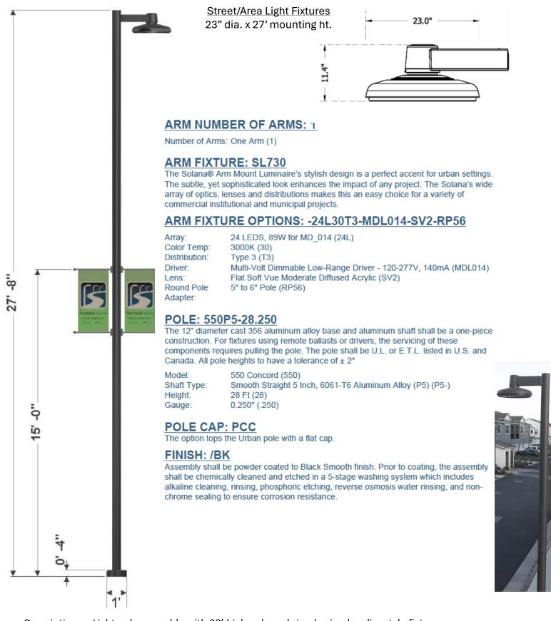
Description: Light pole assembly with 28' high pole and simple circular, disc style fixture Concord pole with Solara arm mount fixture by Sternberg Lighting, <u>www.sternberglighting.com</u>
