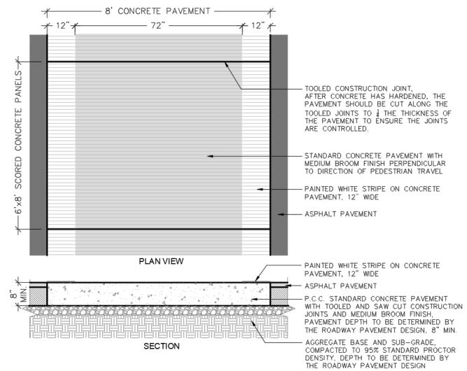
Description: Concrete pavement with tooled joints (8" thick) with painted white stripes (12" wide) Portland Cement, Section 1001 of the IDOT Standard Specifications
