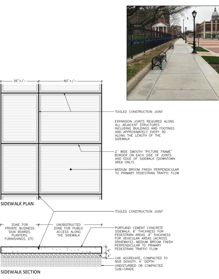
Description: Concrete pavement with tooled joints, 6" thick (pedestrian areas), 8" thick (across driveways) Portland Cement, Section 1001 of the IDOT Standard Specifications
