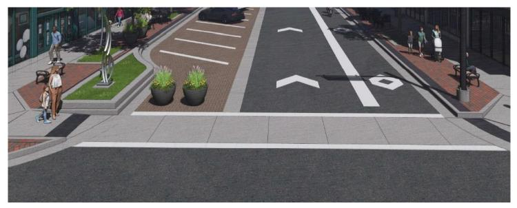
Concrete crosswalk pavement (8' wide) with painted white stripes (12" wide) on each side of the concrete surface to delineate the crosswalk and meet safety standards
